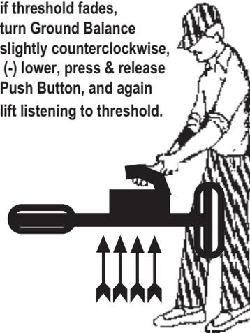
Lift about six inches if threshold increases, turn Ground Balance slightly clockwise, (+) lower, press & release Push Button, and again lift listening to threshold.
