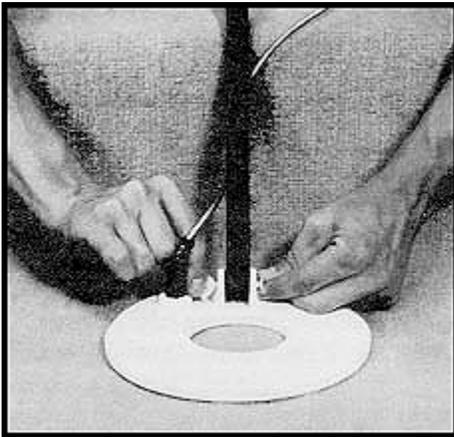
1. On the lower pole assembly, remove the mounting screw and thumb nut from the black nylon pole tip.
