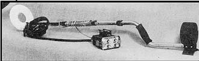
Converting the Tiger Shark from pole mount to body/belt mount is simply a matter of removing the control box from the upper pole and unwinding the cable. To remove the control box from the pole, depress the four spring buttons that hold the mounting bracket and control box to the pole and lift. It is easiest to release one set of spring buttons at a time.
