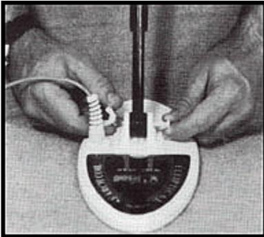
1. Remove the mounting screw and thumb nut from the black nylon pole tip mounted on the end of the lower pole.
