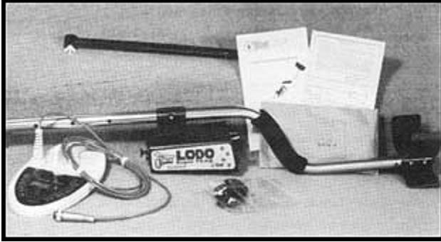
Assembly of the Lobo SuperTRAQ is simple and requires no special tools. Just install the batteries, mount the searchcoil on the lower pole assembly, connect the three pole assemblies, wrap the excess cable around the pole and plug the cable into the control housing. Finally, adjust the pole length and searchcoil angle and you're ready!
