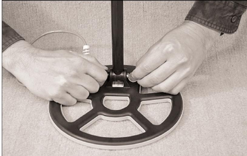
3. Insert the mounting screw through the holes in the mounting ears and pole tip—entering from the side opposite the cable connection.
