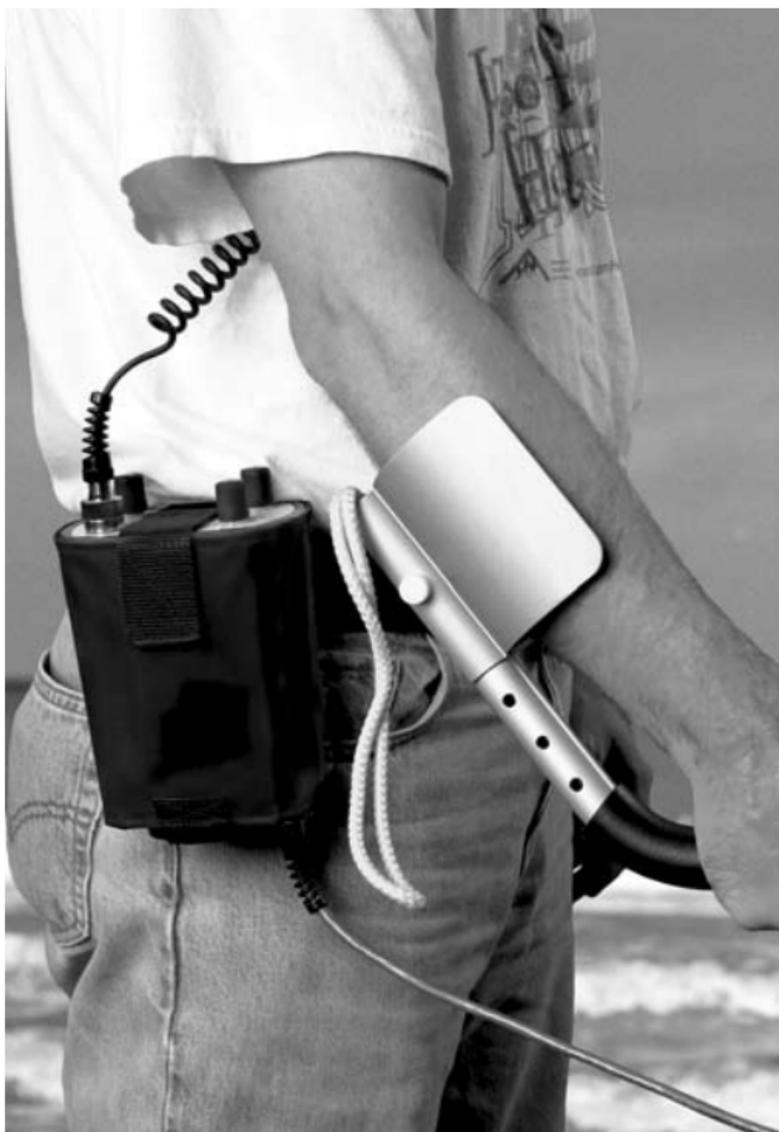
**Figure 5, Long stem with hip mount configurations**
